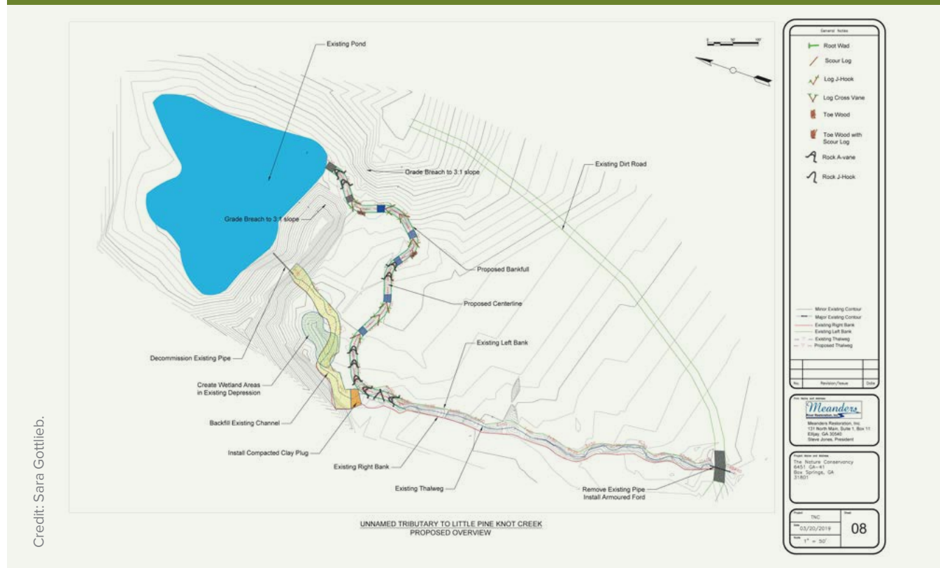
Figure 4: Design for Little Pine Knot dam removal and stream restoration
